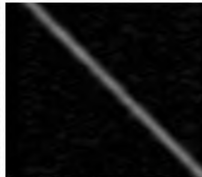
Smoothed derivative removes noise, but blurs edge
